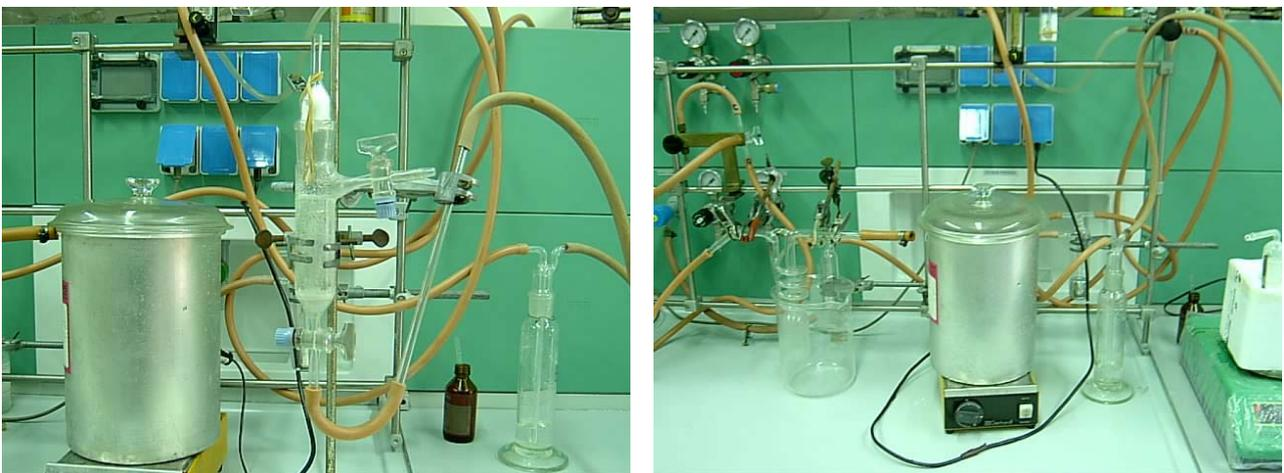
Figure 11 – Laboratory experiment on the use of phosphate for CO<sub>2</sub> removal. Left, absorption bottle; right, close-up of desorber.
